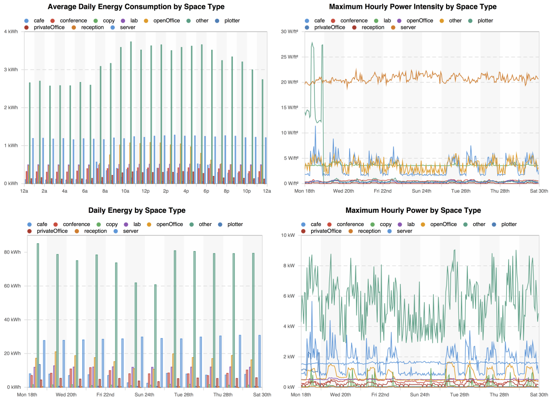
Figure 5.6: Energy and power consumption characteristics grouped by space type June 18th - June 29th, 2018
